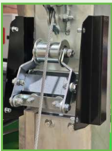
New Safety Feature Emergency Mast Brake
